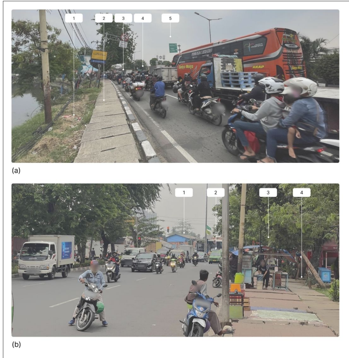
Figure 3. Field walkability observations in front of the Kalideres Terminal highlight several issues: (a1) lack of border separating pedestrian walkways from the Moonkevert river, with unattended urban utilities; (a2) multiuse pedestrian walkway above culverts lacking safety standards; 72 (a3) narrowed pathways causing potential congestion; (a4 and b1) congestion of large buses due to narrowed lanes; (b3) characteristics of local paratransit (angkot); (b3) presence of informal traders/hawkers due to congestion; (b4) narrowing of pedestrian walkways due to hawkers; (b5) signage at Kalideres Terminal.
