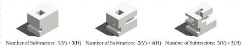
Fig. Generated building massings based on different numbers of subtractors: V indicates vertical subtractors, H indicates horizontal subtractors.
